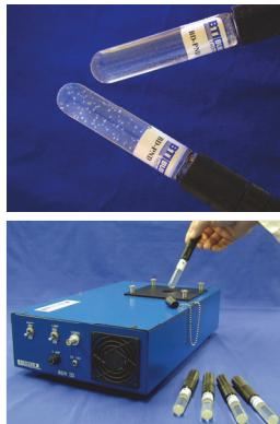
BTI's unique neutron **bubble detectors** are the world's most sensitive and accurate neutron dosimeters. They have been used by nuclear facilities, hospitals, military groups, and space agencies for neutron measurements and **personal neutron dosimetry** for over twenty-five years.
