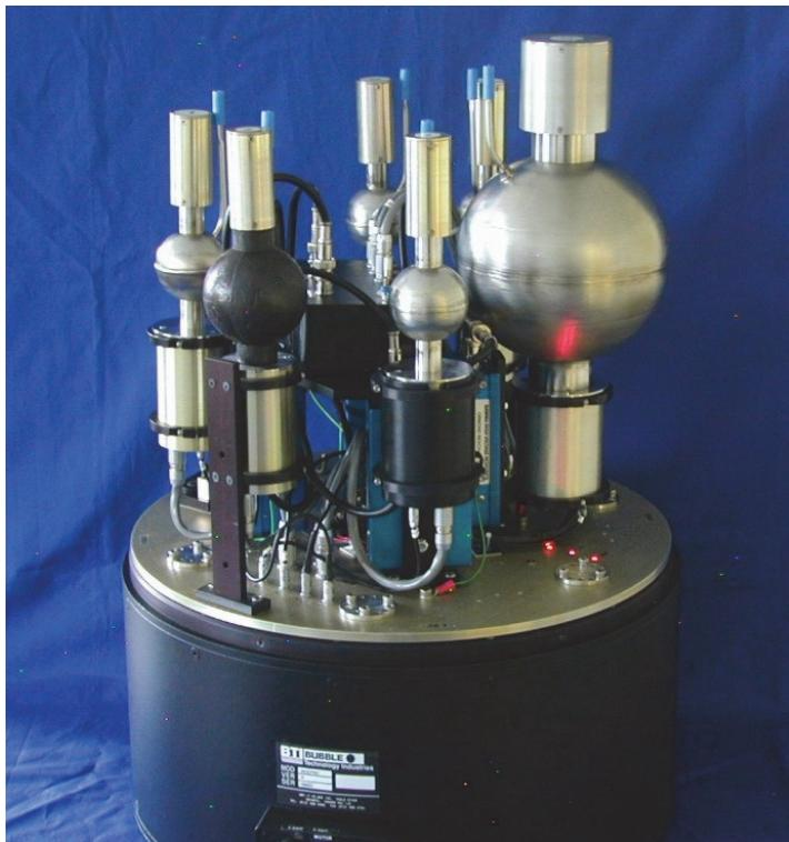
Six (6) detectors cover neutron measurement from the thermal region to 4.5 MeV. System includes four spherical proportional counters with appropriate gas fill for neutron measurements from 50 keV to 4.5 MeV, and two  $^3\text{He}$  detectors for the thermal and epi-thermal region.
