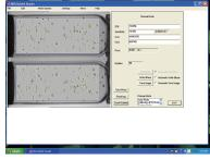
The BDR-III<sup>TM</sup> Automatic Bubble Reader is an affordable solution for automatic counting of large numbers of detectors. The BDR-III provides bar code-ready, fully automated counting with machine vision technology that generates database compatible files in a compact, simple-to-use instrument.
