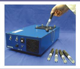
The BDR-III Automatic Bubble Reader is an affordable solution for automatic counting of large numbers of detectors. The BDR-III provides bar code-ready, fully automated counting with USB camera machine vision technology that generates database compatible files in a compact, simple-to-use instrument.
